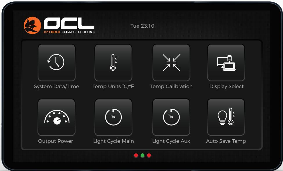
runs a standard cycle that is programmed for a 12H on/12H off schedule. i.e. AUX Environment (R2) turns on after MAIN Environment (R1) turns off and the other way around. AUX Environment (R2) can run a customized schedule autonomous from MAIN Environment (R1) with a Standard 24H Timer or Optimum Time Schedule.
